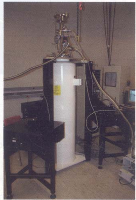
FIGURE 3. The Arizona State University dewar system sits on three Minus K negative-stiffness vibration-isolation systems. The black vertical structures are custom-built mechanical bars that ride on the isolators and support the dewar itself. (Courtesy Arizona State University)
