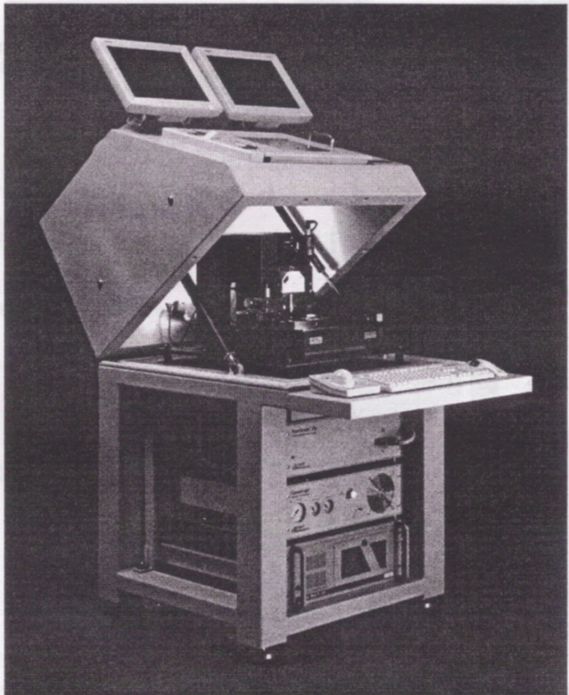
Figure 5 Nano-K™ "Biscuit" NSM Bench Top Vibration Isolation Platform with Digital Instruments Dimension™ 3000 AFM (courtesy of Digital Instruments, Veeco Metrology Group)
